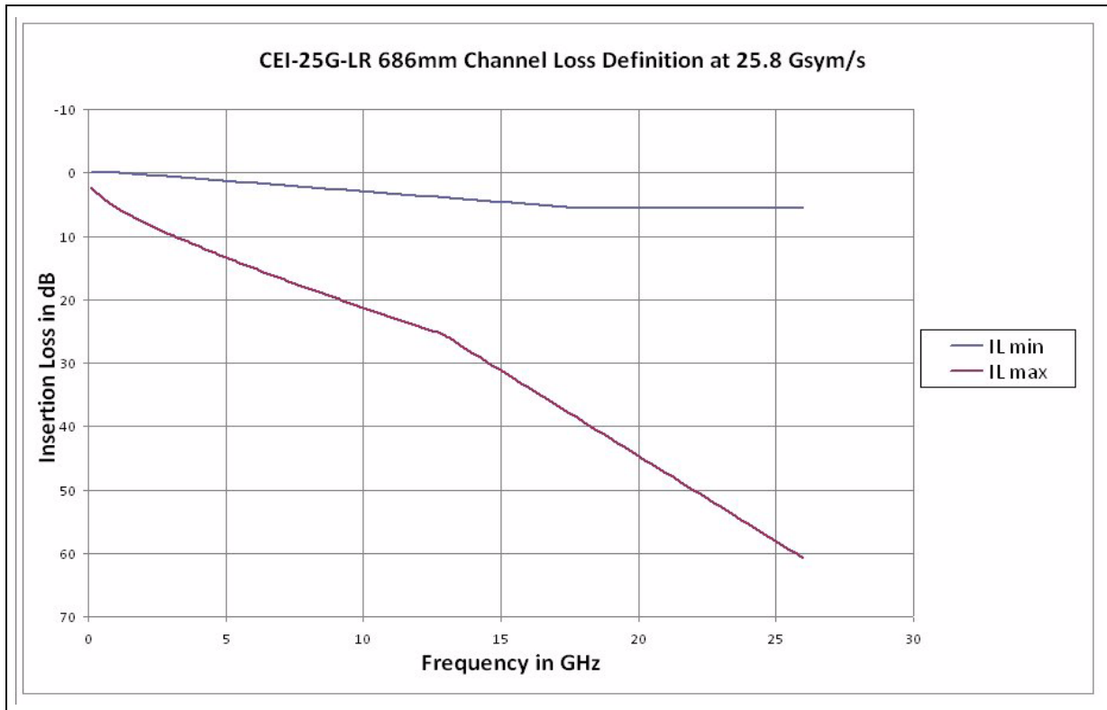
Figure 11-2. CEI-25G-LR Normative Channel Insertion Loss at 25.80 Gsym/s.
